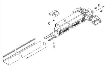
4 Cut new cover plate as needed to match exit device length.
