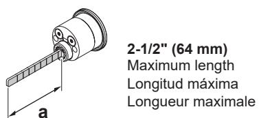
Assemble cylinder to 2-piece cylinder collar
