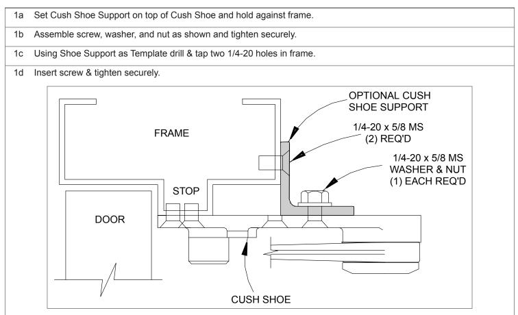
Should frames have 1/2" Blade Stop it is necessary to use 1/2" Blade stop Spacer (available from Dealer). Use both Blade Stop Spacer and Shoe Support wherever required.
