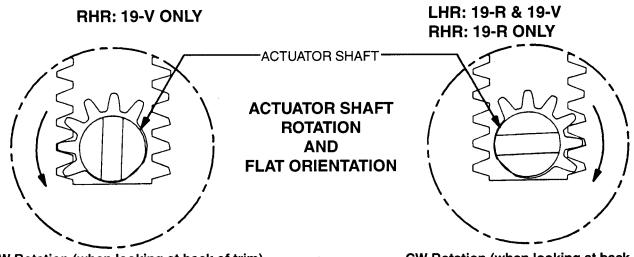
**CCW Rotation (when looking at back of trim)** Gear teeth meshed as shown with flats in horizontal position.
