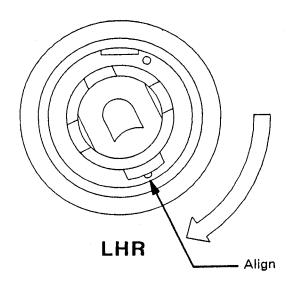
4. SELECT PROPER SPRING AND SLIDE SPRING OVER SPINDLE, THEN INSERT STRAIGHT "LEG" OF SPRING INTO SPRING LOCATOR HOLE.
