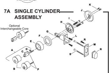
Single Cylinder Screw 1/4" bolts (I) through plate\* (H) into housing (B) & tighten. Engage tailpiece (P) with thumbturn (J). Fasten thumbturn (J) to plate (H) with short machine screws (K)
