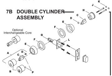
Screw 1/4" bolts (J) through housing (H), **Double Cylinder** and ring (E) into housing (B) engaging tailpieces (P) with the vertical slot in the deadbolt
