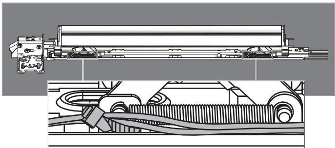
**F** Route and secure wires through center case.
