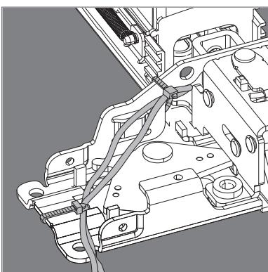
① Note: based on mounting orientation, secure wires through the top side of the centercase.
