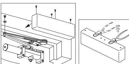
Attach cover with screws and plugs.
