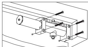
Valves UP for right hand door (shown). Valves DOWN for left
