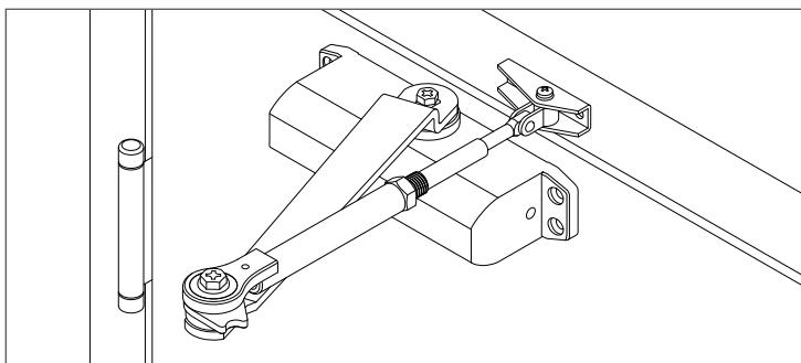
Closer mounted on the pull side of the door (hinge side). Page 3.
