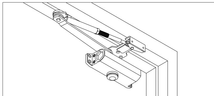
Closer mounted on the push side of the door (opposite of the hinge side). Page 5.
