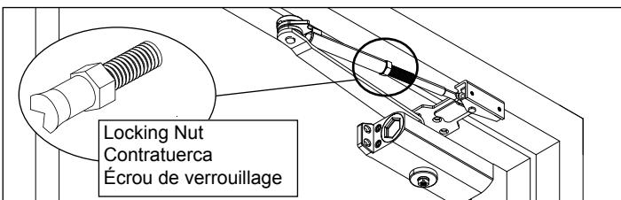
Rotate shaft 45° with wrench before placing arm on top of shaft.
