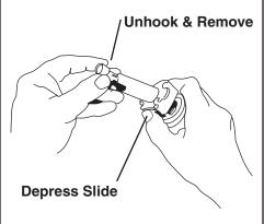
6. Insert new plunger bar (less button assembly), depress slide and push plunger bar while releasing slide to hook into place.
