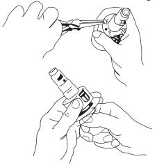
Install new spindle over bar, rotate slightly and push into place. (Slot on spindle should be on same side as slide jaws.)
