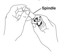
8. Align plunger button assembly so lug fits into slot on spindle. Position plunger button assembly onto bar and snap firmly into place.
