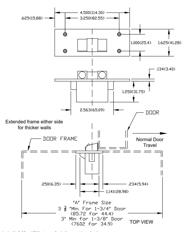
Packed with 8-32 x 1/2" fasteners for hollow metal applications.
