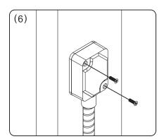
Mount the head covers and tighten the screws.
