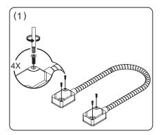
Remove the security screws using the enclosed tool.
