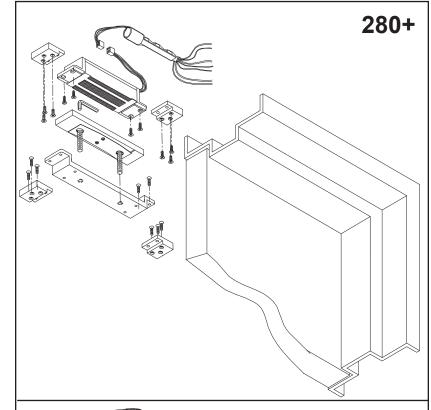
280+ TRD model is a concealed electromagnetic shear lock designed to fit a Aluminum top rail glass doors and open channel hollow metal doors and hollow metal or aluminum frames. It is generally used in cases where the top of the door is not accessible for adjustment. The gap between the armature (in the door) and the magnet (in the frame) is adjusted from the edge of the top rail, through an access hole, with a nut driver or standard screwdriver.
