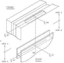
**DOOR STATUS SWITCH:** This MUST be installed for proper operation. It is best installed as close to the latch side (opposite the hinge side) as possible. The switch indicates to the module that the door is in the closet position so it can lock and engage properly.
