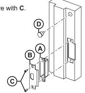
After strike components have been installed, refer to illustration on right & assemble lock components onto door in following order:
