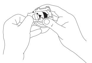
**11.** Place new bar (less button assembly) into position thru splindle and into lock frame. Make sure that bar engages keyway in outside spindle.
