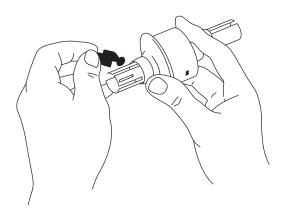
**13.** Slide new knob onto spindle, depress knob catch, and push knob into place until knob catch engages in slot on knob.
