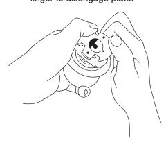
7. Remove slide and springs. If necessary to remove outside hub plate, rotate knob 180° to remove turn and pull outside knob and spindle from lock frame. Unhook & Remove
