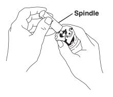
**8.** Align plunger button assembly so lug fits into slot on spindle. Position plunger button assembly onto bar and snap firmly into place.
