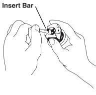
7. Install new spindle over bar, rotate slightly and push into place. (Slot on spindle should be on same side as slide jaws.)
