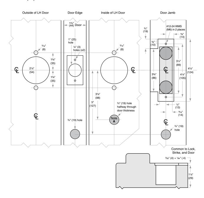
Dimensions shown in parentheses () are in millimeters.
