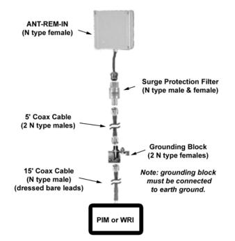
Figure 6-2 - ANT-REM-IN Recommended Protection
