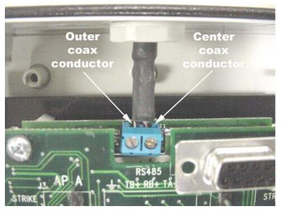
Figure 6-14 – PIM PCB Antenna Terminal Block Connections
