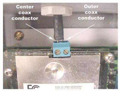
Figure 6-22 – WRI-OTD-12VDC PCB Antenna Terminal Block Connections
