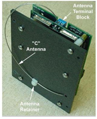
Figure 6-10 – Removing the PIM's Internal "C" Antenna
