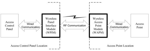
Figure 1-1 – Schlage Wireless<sup>TM</sup> Access System Block Diagram
