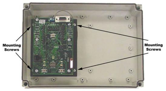
Figure 6-9 – Removing PIM PCB
