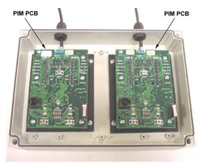
Figure 6-8 – PIM-TD4 with RAMs Installed
