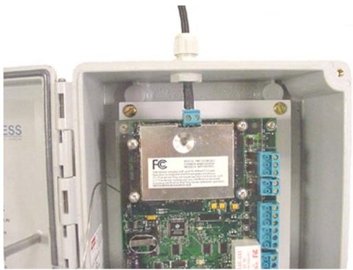
Figure 6-21 – Installing the RAM Coax in the WRI-OTD-12VDC
