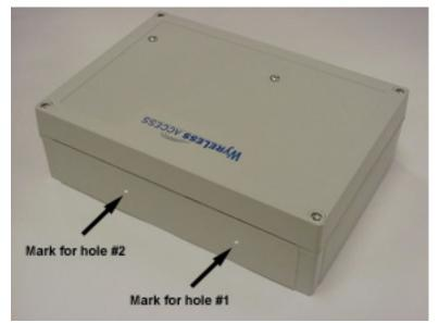
Figure 6-11 – PIM Antenna Hole Locations
