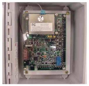
Figure 6-16 – Removing the WRI-OTD-12VDC PCB
