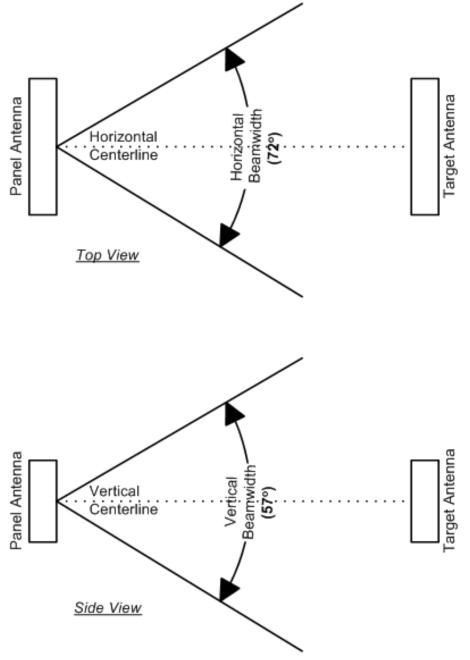
Figure 5-2 - ANT-REM-I/O+6DB RF Radiation Pattern
