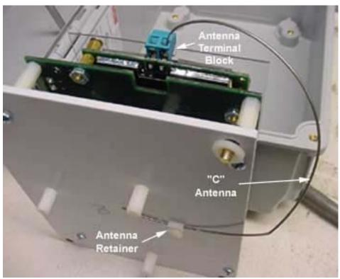
Figure 6-17 – Removing the WRI-OTD-12VDC's Internal "C" Antenna
