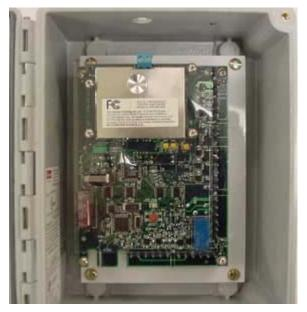
Figure 6-19 – Replacing the WRI-OTD-12VDC's PCB
