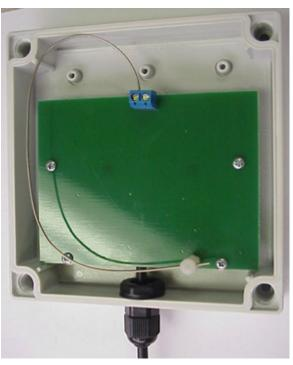
Figure 3-1 – ANT-REM-IN with Cover Removed
