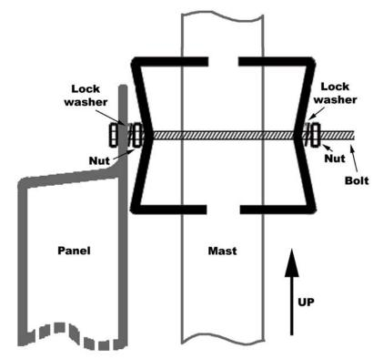
Figure 5-3 – Mast Mounting Clamp Installation
