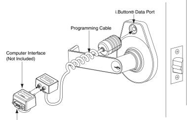
For 9-Pin Cable connection to computer
