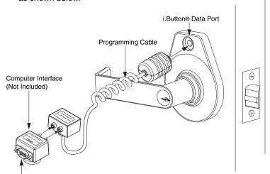
For 9-Pin Cable connection to computer
