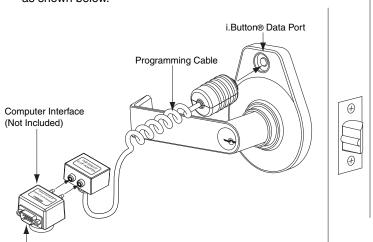
For 9-Pin Cable connection to computer
