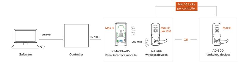
AD-400 wireless range up to 200' in typical building construction, up to 1000' line of sight.
