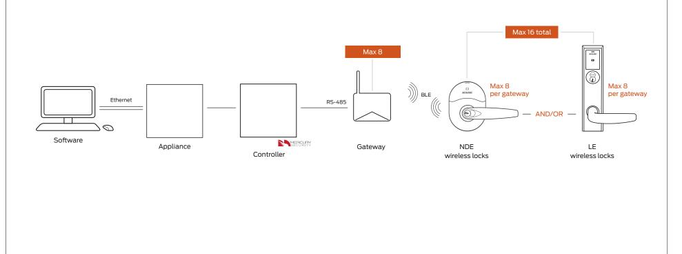
Gateway communication range up to 30' in typical building environments; a detailed site survey is recommended.
