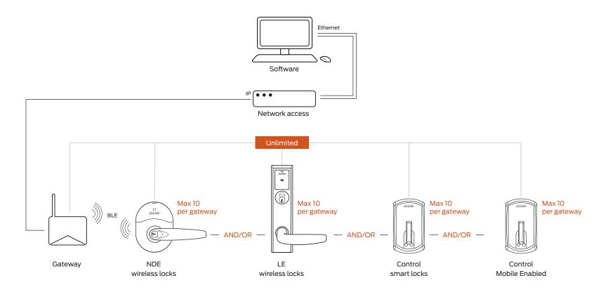
Gateway communication range up to 30' in typical building environments; a detailed site survey is recommended.
