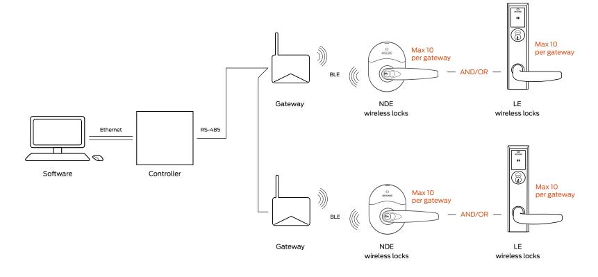
Gateway communication range up to 30' in typical building environments; a detailed site survey is recommended.
