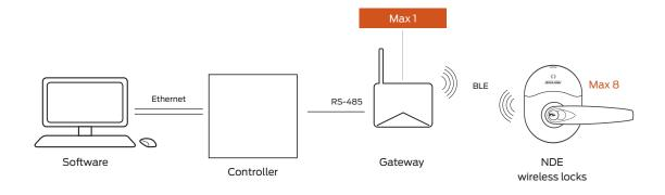
Gateway communication range up to 30' in typical building environments; a detailed site survey is recommended.
