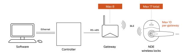
Gateway communication range up to 30' in typical building environments; a detailed site survey is recommended.
