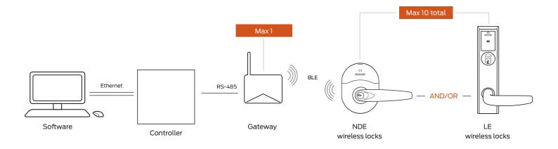
Gateway communication range up to 30' in typical building environments; a detailed site survey is recommended.
