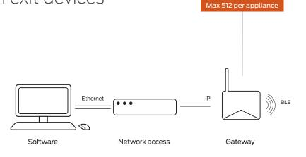
per gateway wireless locks AND/OR Max 10 per gateway LE/B wireless locks Max 2,048 total per appliance AND/OR Max 10 per gateway Control/Control mobile enabled smart locks AND/OR Exit devices with RU/RM option
