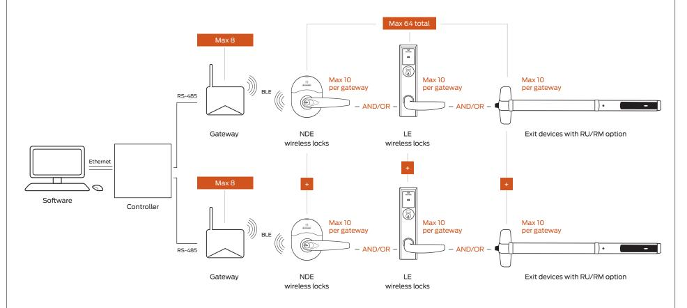
Gateway communication range up to 30' in typical building environments; a detailed site survey is recommended.
