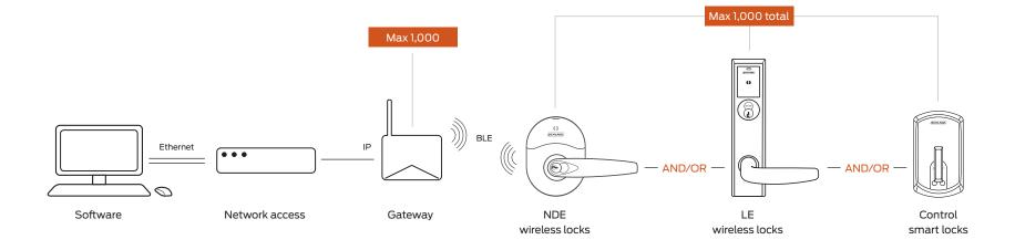
Gateway communication range up to 30' in typical building environments; a detailed site survey is recommended.
