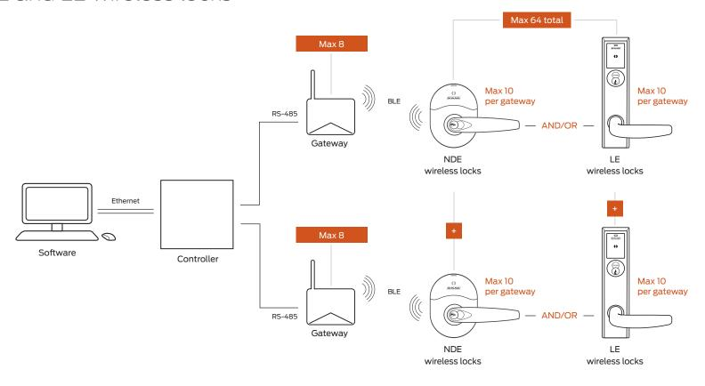
Gateway communication range up to 30' in typical building environments; a detailed site survey is recommended.
