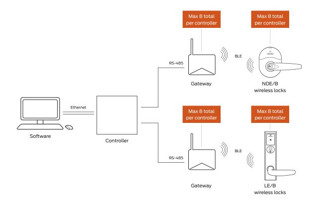
Gateway communication range up to 30' in typical building environments; a detailed site survey is recommended.
