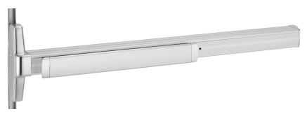
3347A and 3547A for all types of single and double doors, UL listed for panic exit hardware. Devices are ANSI A156.3 - 2008 Grade 1. The 3547A has a smooth mechanism case and the 3347A has grooved case. The concealed vertical rod device is non-handed except when the SS (signal switch) option is used.
