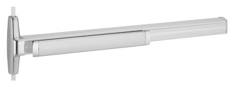
3327A-F and 3527A-F for all types of double doors up to 8' x 10' (2438mm x 2540mm), UL listed for Fire Exit Hardware. See Additional information section of the catatog for detailed information on UL listed fire exit hardware label and door opening size information. Devices are ANSI A156.3 - 2008 Grade 1. The 3527A-F has a smooth mechanism case and the 3327A-F has grooved case. The surface vertical rod device is non-handed except when the SS (Signal Switch) option is used.
