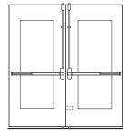
Two fire exit hardware vertical cables/rods with auxilary fire latch-LBR option\*
