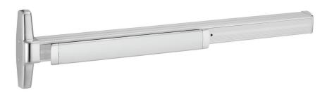
**3349A** and **3549A** for hollow metal single and double doors, UL listed for panic exit hardware. Devices are ANSI A156.3 – 2008 (LBL option 2014) Grade 1. The 3549A has a smooth mechanism case and the 3349A has grooved case. The concealed vertical cable device is non-handed except when the SS (signal switch) option is used.
