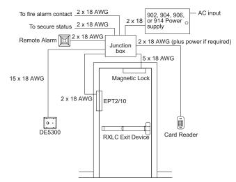
Figure 1. Riser diagram, single door
