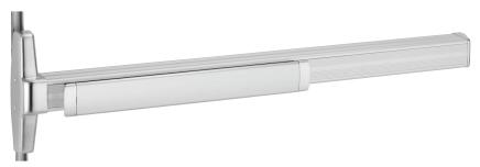
3348A and 3548A for hollow metal single and double doors, UL listed for panic exit hardware. Devices are ANSI A156.3 – 2008 Grade 1. The 3548A has a smooth mechanism case and the 3348A has grooved case. The concealed vertical rod device is non-handed except when the SS (Signal Switch) option is used.
