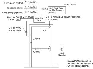
Figure 1. Riser diagram, single door
