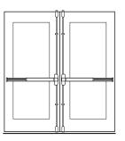
Two surface mounted vertical rod devices-same direction\*
