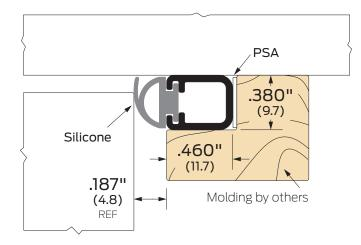
Notes: Extruded Bulb/Finger for double-sealing protection. Supplied standard with PSA.
