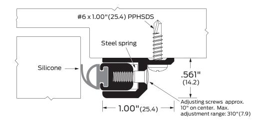
Notes: Adjustable and spring loaded. Extruded Bulb/Finger for double-sealing protection.
