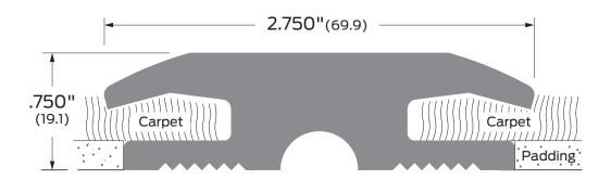
Notes: Traction Tread™ rubber for non-rated door. Supplied without mounting holes.
