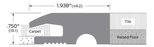
Notes: Traction Tread<sup>™</sup> rubber for non-rated door. Supplied without mounting holes.
